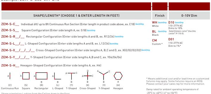
Shape orientation Looking from the Ceiling down to the floor. All corners of shape must be 90° or 120°, same plane, joiners and rolling lens will be included FOR more complex shape, CONTACT OKT.
